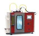
Tannas Foam *Air* Bath (TFAB<sup>™</sup>) • ASTM D892, D6082, IP146 • Non-liquid bath • 24°C to 150°C range
